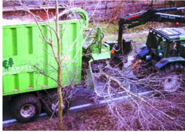
A mobile chipper with crane efficiently collects roadside thinnings for fuel. (Courtesy of Bruins and Kwast, Netherlands)
