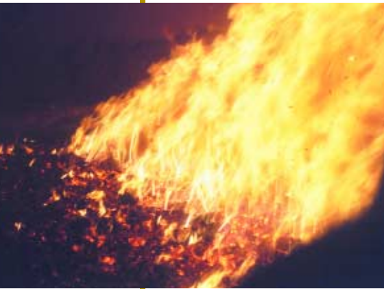
Wood chip combustion on a grate furnace. Fuel enters the furnace at the right hand side and devolatilizes as it is transported to the left. At the left hand side, remaining char burns out.
