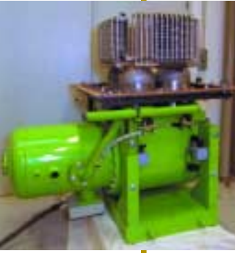
35 kW e Stirling engine for biomass combustion plants. (Courtesy of Henrik Carlsen, Denmark)
