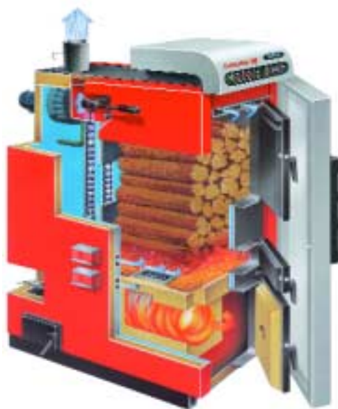
A microprocessor controlled woodlog stove with downdraught combustion and separate chamber where secondary combustion takes place. (Courtesy of Fröling, Austria)
