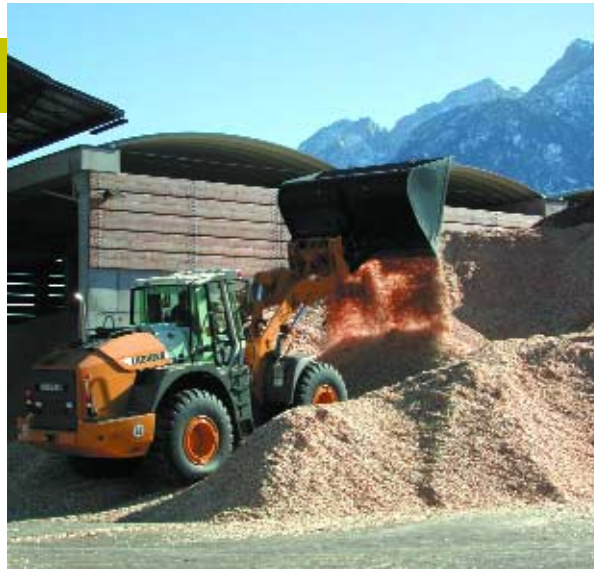
Wheel loaders are often used for transporting sawdust and bark from the long-term storage to the feeding system of the biomass heating plant. (Courtesy of Stadtwärme Linz, Austria)
